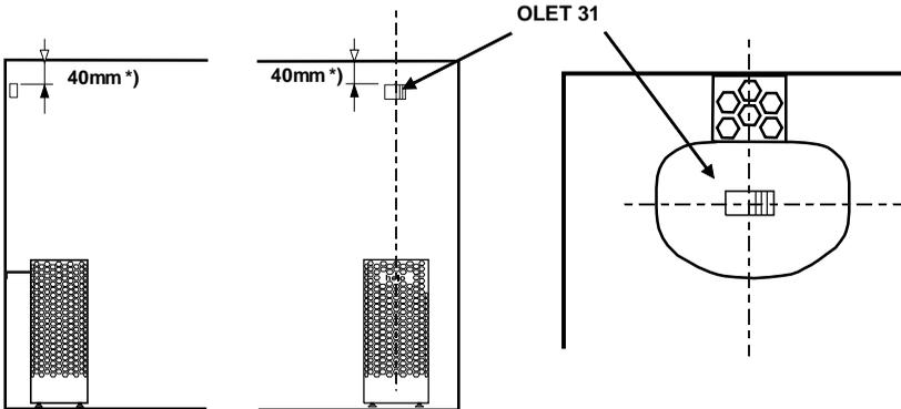
Abbildung 2. Sensor OLET 31 installation location on the wall
